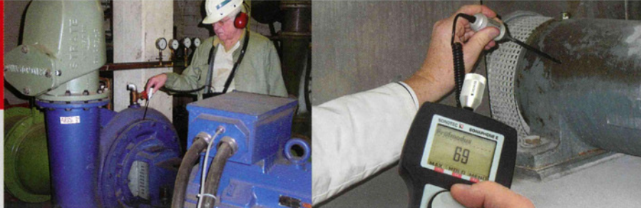
First signs of wear in sliding or rolling bearings are easily detected using body sound detection technology.
